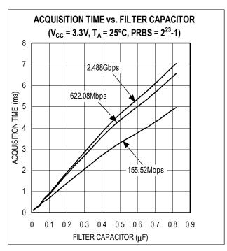
Figure 7. Acquisition Time vs. Filter Capacitor
