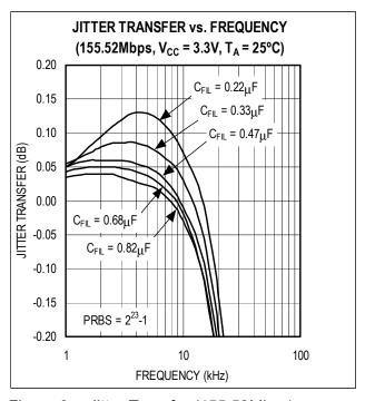
Figure 6. Jitter Transfer (155.52Mbps)
