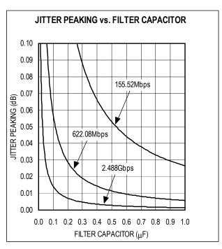
Figure 2. Jitter Peaking vs. Filter Capacitor
