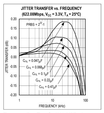
Figure 5. Jitter Transfer (622.08Mbps)
